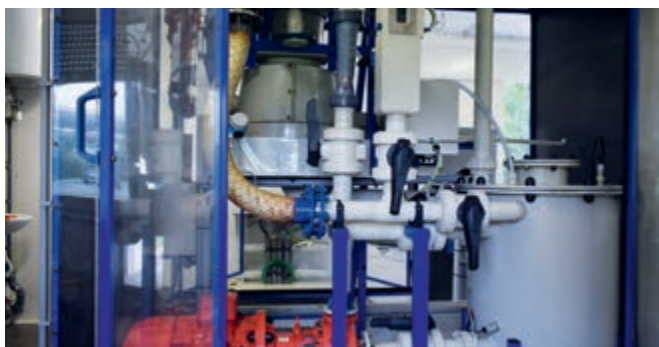
FIG. 3: The simulator comprises an acid tank (to the right), a pump (in red), and an acid chamber (top).
