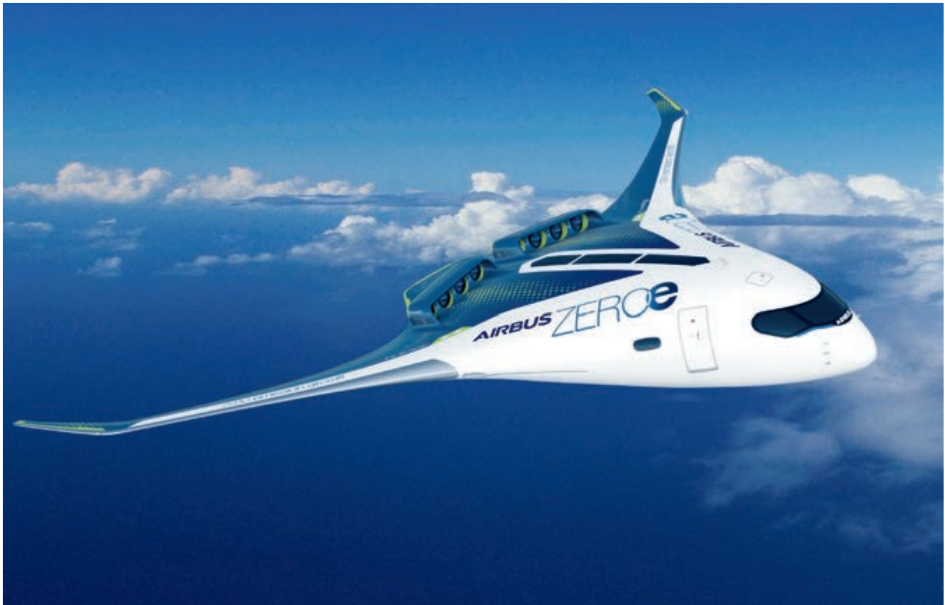
FIG. 2: Airbus has thus far unveiled three hydrogen-powered plane concepts. The futuristic blended-wing version (pictured) could fly up to 200 passengers distances of 2,000 miles.
