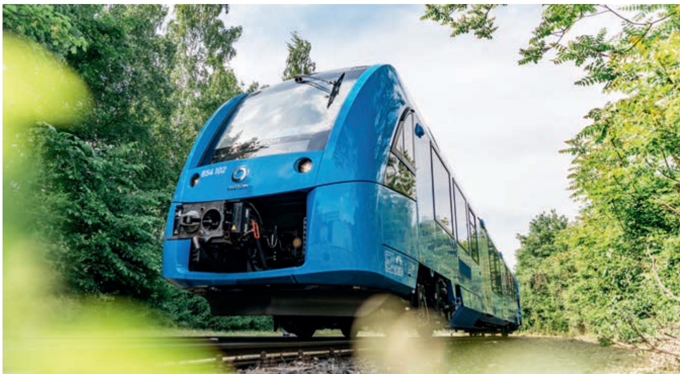
FIG. 1: The zero-emission Coradia iLint is the world's first hydrogen fuel cell-powered passenger train, and winner of the prestigious GreenTec Mobility Award in 2018.
