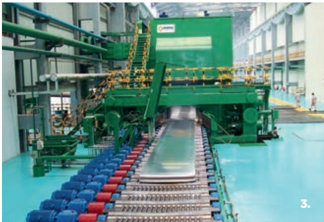
FIG. 2: Ulsan Aluminium 3-stand tandem hot finishing mill. Ulsan produces high-grade automotive coils for Korea's key vehicle manufacturers.
