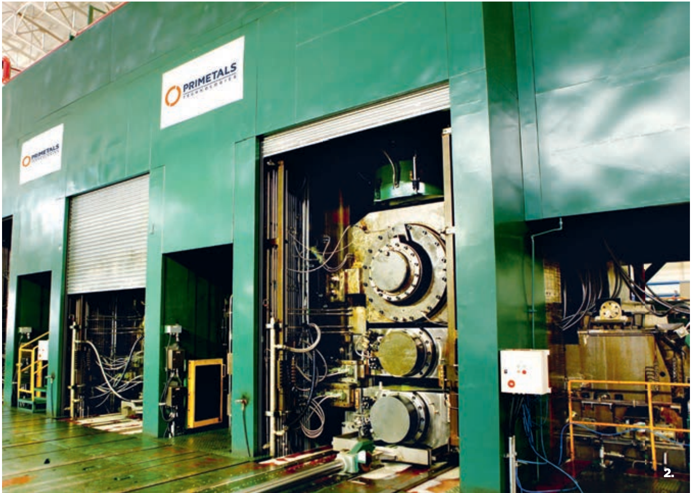
FIG. 2: Ulsan Aluminium 3-stand tandem hot finishing mill. Ulsan produces high-grade automotive coils for Korea's key vehicle manufacturers.
