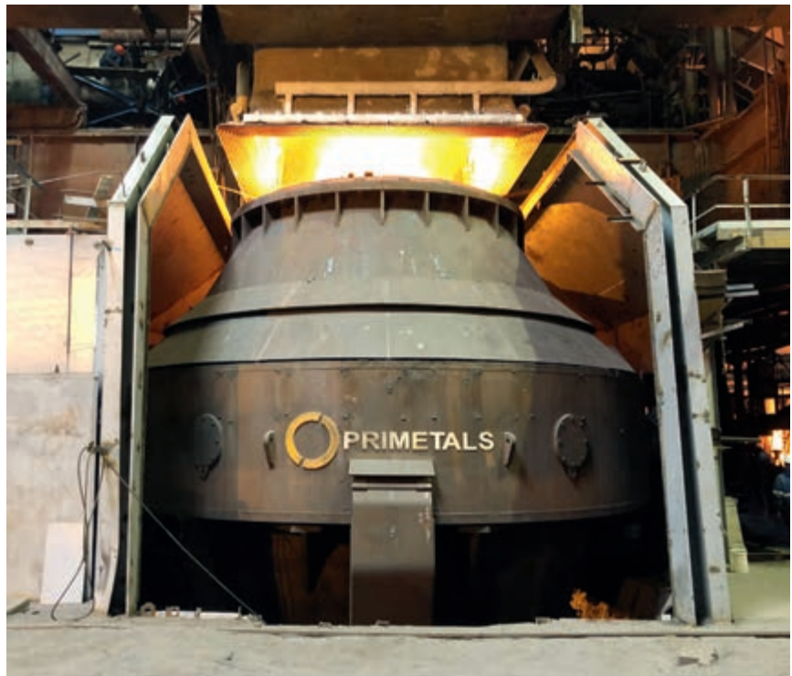
Mechel Group has successfully had its third LD converter (BOF) modernized at the company's Chelyabinsk Metallurgical Plant.
