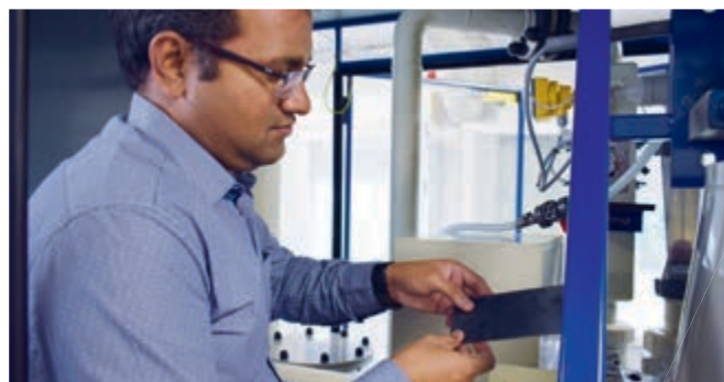
FIG. 4: The simulator uses samples of steel strip to compare traditional pickling methods with the newly developed one.
