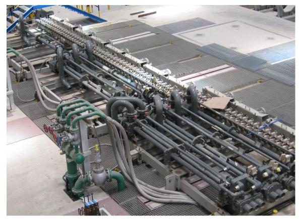
Pomini Quenching System (PQS) for multi-slit operation from Primetals Technologies. The quenching system produces the required material properties largely without the need for expensive alloying elements.
