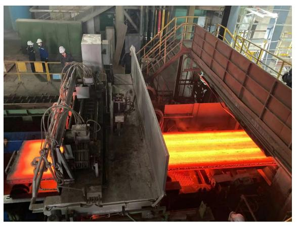
Startup of continuous casting machine CCM4 modernized by Primetals Technologies at Angang Iron & Steel
